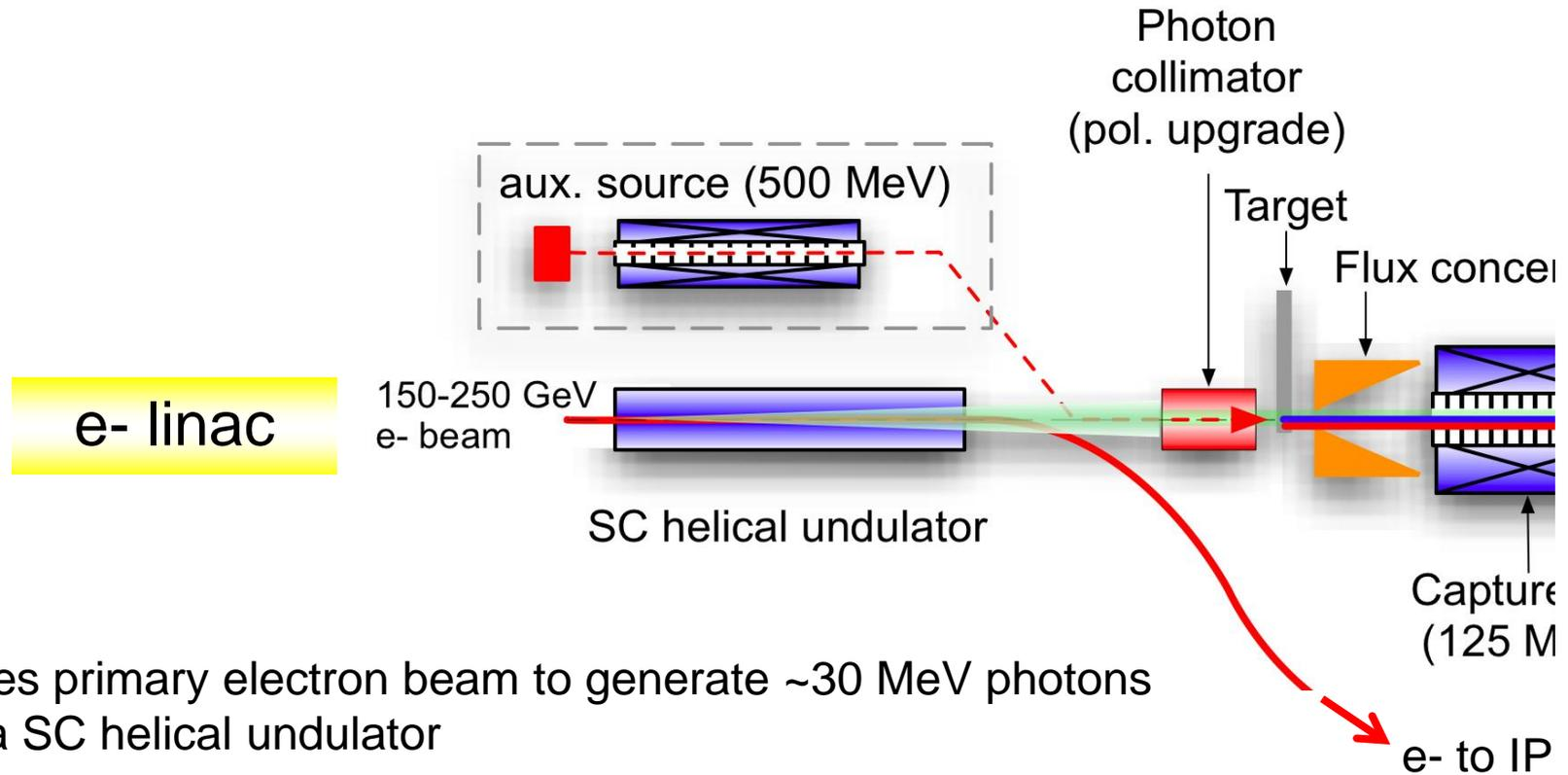
Uses primary electron beam to generate  $\sim 30$  MeV photons in a SC helical undulator
